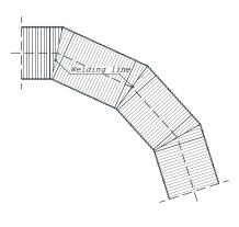
Fig. 5. End finishes in longitudinal section
