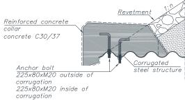
Fig. 7. Example of a concrete collar
